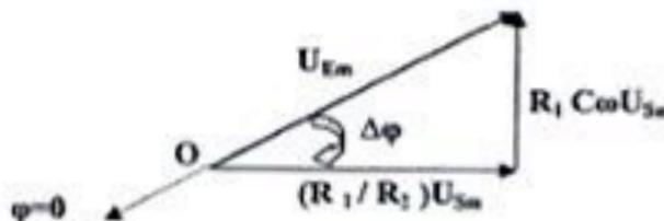
$(U_{Em})^2 = \left(\frac{R_1}{R_2}\right)^2 U_{Sm}^2 + (2\pi N R_1 C)^2 U_{Sm}^2$ <p>Par la suite on a :</p> $T = \frac{1}{\sqrt{\left(\frac{R_1}{R_2}\right)^2 + (2\pi N R_1 C)^2}} = \left(\frac{R_2}{R_1}\right) \cdot \frac{1}{\sqrt{1 + (2\pi N R_2 C)^2}}$ | 0,25x3 |
